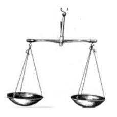
It is used to weigh small amounts of substance: usually 0.06 g - 100-200 g, several weighing models are known of 0.25- 0.5- 1- 2- 5- 10 - 20 g (with the sensitivity decreasing).
