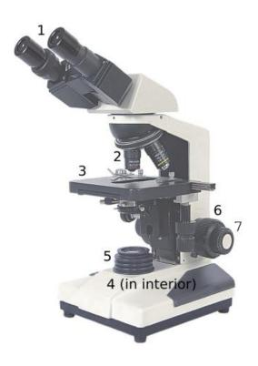
Ocular (1) – contains the lenses ocular; typical magnification values: 5x, 10x and 2x **Objective** (2); typical values of magnifications: 4x, 5x, 10x, 20x, 40x, 50x and 100x; interchangeable **Table** (3) – supports the test of examination **Light source** (4) – located under the table **Condenser** (5) – system of lenses and diaphragms which controls the amount of light by focusing the light **Macrovisa** (6) and **microvisa** (7) used to clarify image
