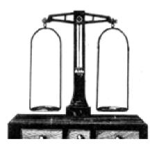
It is used in the pharmacy to weigh from 10 to 1000g or from 5 to 500g with a sensitivity of centigrams.
