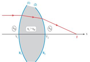
If the light consecutively pierces two spherical diopters and the space between these diopters has a different refractive index than that outside, then the pair of diopters forms a "lens".
