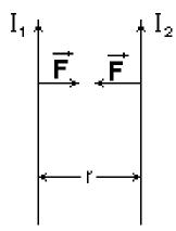
Picture: 63: Reciprocal action between two conductors through which an electric current passes
