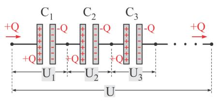
Figure 18: Capacitors connected in series
