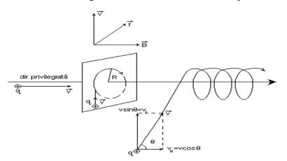
Figure 50: The movement of a particle in a magnetic field
