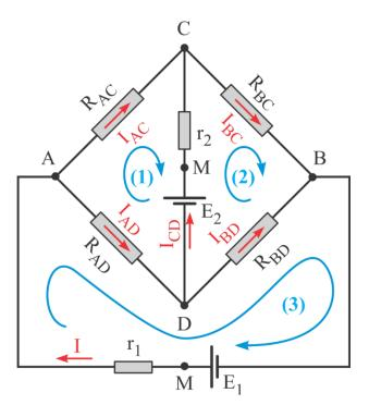
Figure 35: Analysis of the circuits traversed by the direct current
