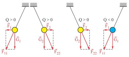
Figure 1: Electric forces and charges
