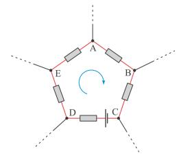
Figure 33: The circuit through which the direct current flows.
