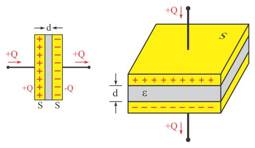
Figure 16: The electrical capacity of a capacitor
