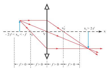
If the real object is between the distances of 2  $\cdot$ f and f with respect to the lens (- 2  $\cdot$  f <xo <f), then the image is real, inverted, magnified in comparison with the object and shape at a distance greater than 2  $\cdot$  f from the lens.
