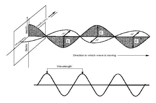
Figure 86: Electromagnetic waves in vacuum
