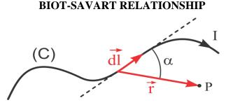
Figure 52: The magnetic induction vector  $(B_P)$  produced in the point P by the current in the infinitesimal part of the conductor (dl),
