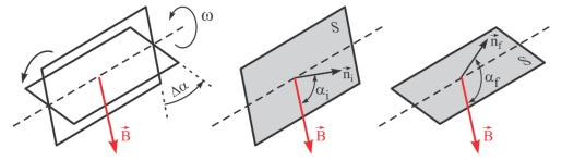
Figure 77: The direction of the electromotive voltage of the current
