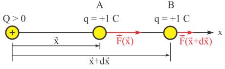
Figure 9: Electric charges and forces (Q>0)
