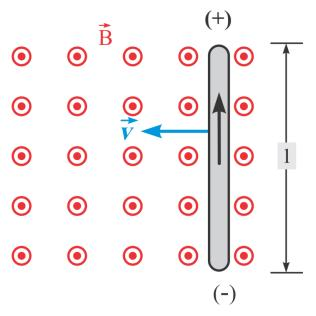
Figure 75: The direction of the electromotive voltage of the current
