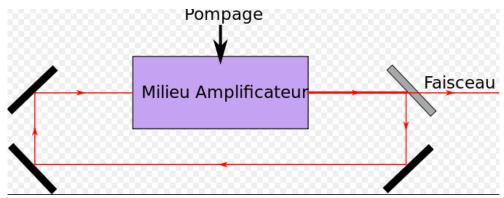
Figure 96: Laser operating principle
