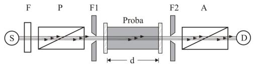
Details for the construction of a conventional polarimeter (l): the resonance radiation of Na vapors - 589.3 nm
