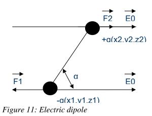
The electric dipole supports the action of a couple of forces whose value is:  $C = \frac{F_2}{\sin \alpha}$   $\vec{C} = \vec{p} \times \vec{E}_o$
