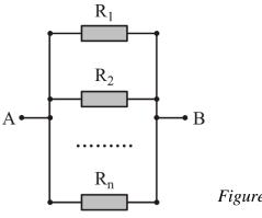
Figure 28: Resistors in parallel:
