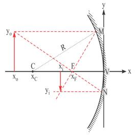
If the object is located further than the radius of the spherical mirror "R" from the point "V", then the concave mirror gives a real, inverted and diminished image (relative to the object).
