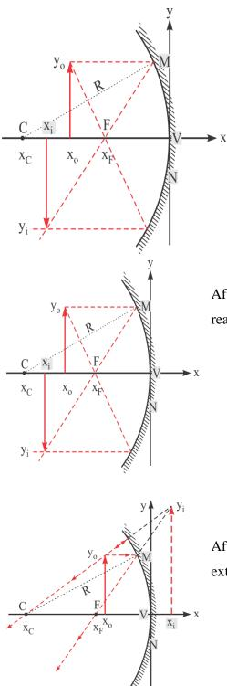
If the object is located between the center and the focus of the spherical mirror, then the concave mirror gives a real image, reversed and magnified (relative to the object). If the object is located in the center of the spherical mirror,
