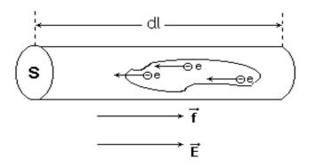
Figure: 62: The force acting in a magnetic field on a conductor through which an electric current passes
