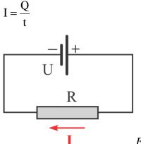
Figure 24: Electric circuit traversed by a current of intensity I
