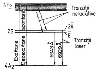
In the Figure are schematically represented ruby energy levels involved in this effect, using spectroscopic notations
