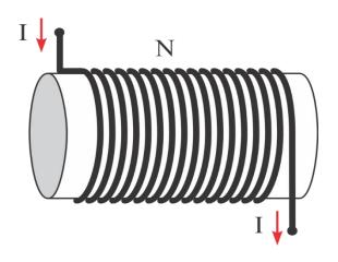
Figure 54: Magnetic induction inside a solenoid
