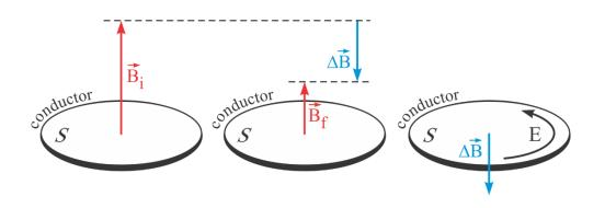
Figure 73: Electromotive voltage induced by time variation of magnetic induction
