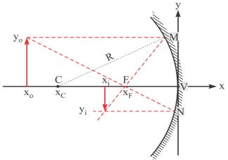
The Physical quantities involved refer to a system of axes (xOy) which originates from the starting point "V" of the spherical mirror.
