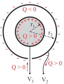
Figure 17: The electrical capacity of a spherical conductor
