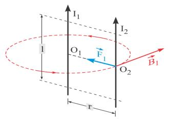
Figure: 64: Magnetic interaction of electric currents
