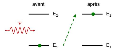
Figure 94: Laser operating principle
