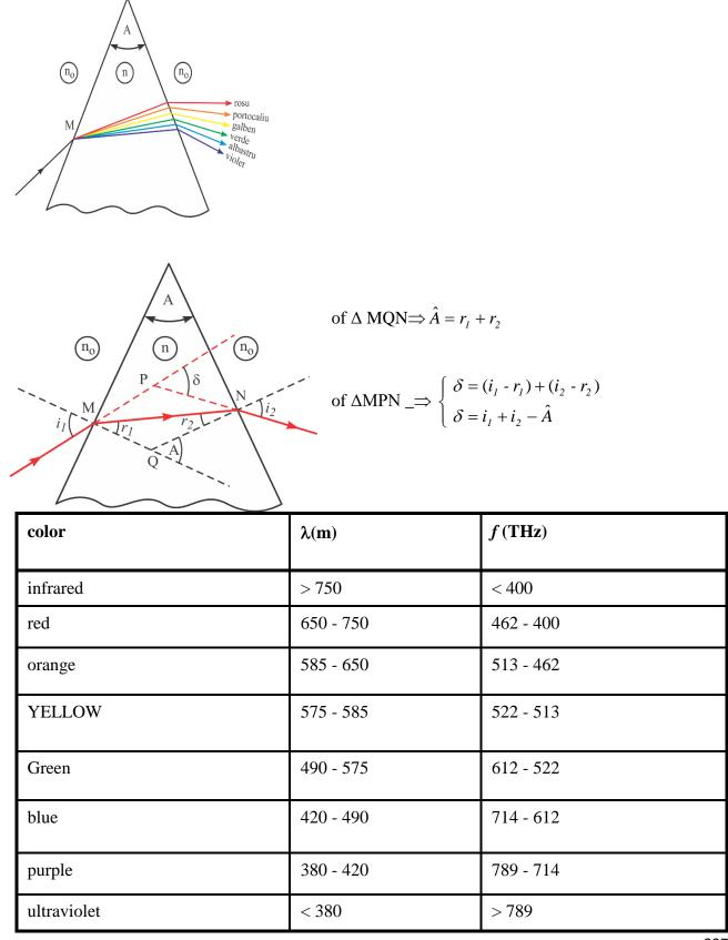
The refractive index in optical media depends on the wavelength of the incident light (this is the phenomenon of dispersion). White light is a mixture of components at different wavelengths. Therefore, when white light is incident on the emergent surface, the direction of propagation depends on the wavelength of the components.
