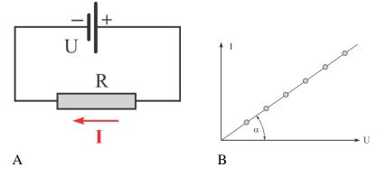
Figure 25:A) the simple electrical circuit; B) the representation of Ohm's law.
