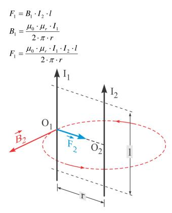
Figure: 65: Magnetic interaction of electric currents
