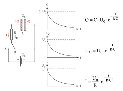
Figure 21: Discharging a capacitor
