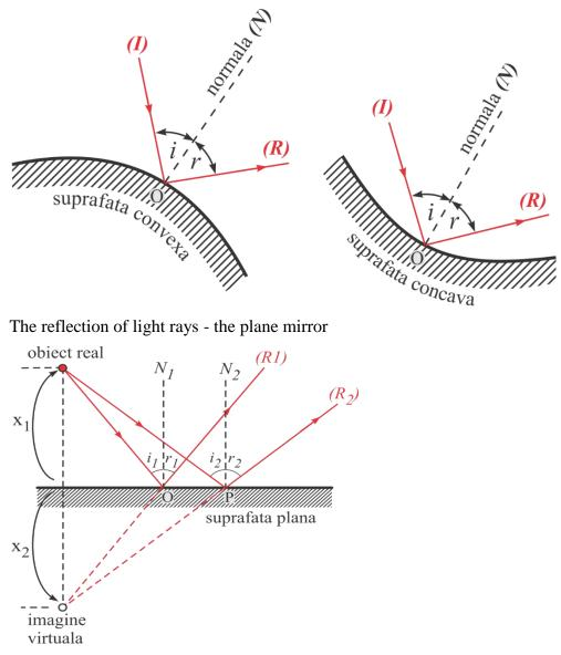
The light rays which propagate from a punctiform source (a real object) diverge, after undergoing reflection on a plane surface. They do not intersect, but their extensions come together in a point (virtual image).
