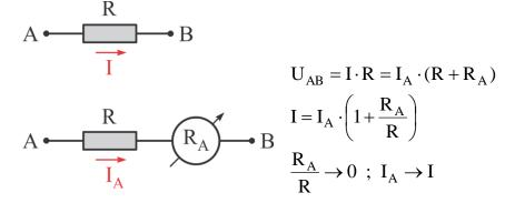
Figure 29: Measurement of current intensity in a circuit with The ideal ammeter
