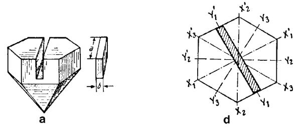
The quartz blade is cut along a direction perpendicular to an X axis ("X" cut) and subjected to a compression along the corresponding Y axis, its faces (perpendicular to X) different electrification, one positive and the other negative.
