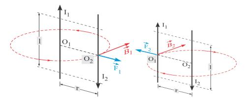
Figure: 67: Magnetic interaction of electric currents
