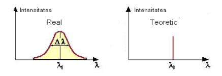
Figure 97: properties of laser radiation
