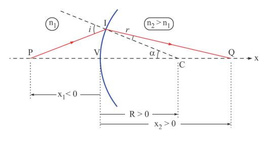
Sine theorem for  $\triangle PIC$ :  $\frac{PC}{\sin(\pi - i)} = \frac{PI}{\sin \alpha}$  and  $\frac{-x_1 + R}{\sin i} = \frac{-x_1}{\sin \alpha}$
