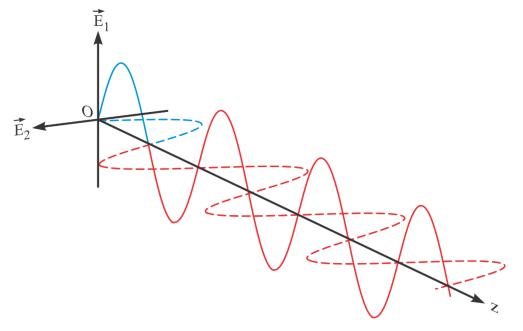
The vector sum of the intensities of the electric fields is, in each moment, a wave always linearly polarized (result: a linearly polarized wave).
