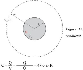
Figure 15: The electrical capacitance of a spherical conductor
