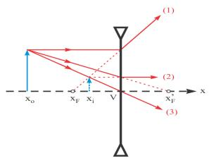
At any position of the real object, the diverging lenses form an image only at the prolonged intersection of the real rays.
