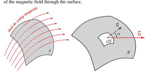
Figure 68: Magnetic flux relative to a surface
