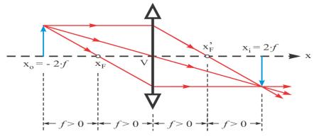
If the real object is at the distance of 2 •f with respect to the lens (xo = 2 • f), then the image is real, inverted, of the same size with the object and is formed at the distance 2 •f with respect to the lens.
