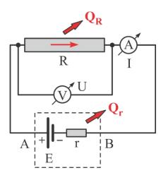
Figure 37: The heat dissipation  $(Q_R)$  on R of external resistance
