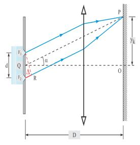
The optical path difference between the two directions D From the triangle F<sub>1</sub>F<sub>2</sub>R:  $\Delta = d \cdot \sin \alpha$ Condition of maximum illumination at point P:  $\Delta = d \cdot \sin \alpha = k \cdot \lambda$  and  $tg\alpha = \frac{y_k}{D}$ From triangle OPQ:  $y_k = D \cdot tg\alpha$ If a < 3°, then  $tg\alpha \approx \sin \alpha$ We have :  $y_k = D \cdot \frac{k \cdot \lambda}{d}$ y<sub>k</sub> is the "y" axis of maximum illumination of order "k"
