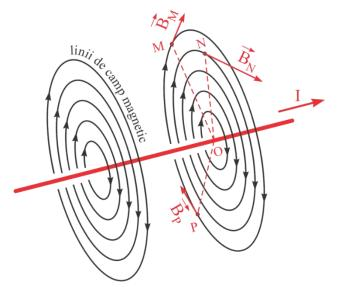
Figure 49: Magnetic field lines
