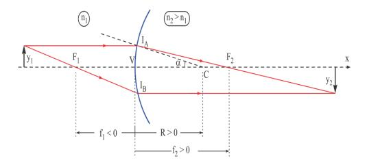
The object-dioptre distance is greater than the distance corresponding to point F1 (object focus).
