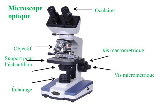
The microscope is an optical instrument that gives a much magnified image of an object, thus making it possible to distinguish details that are not visible to the naked eye.
