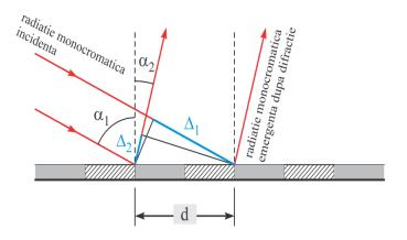
The diffraction grating in reflection: the reflective and opaque parts are alternated.
