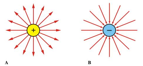
Figure 6: A: The field lines of a positive point-like charge; B: Field lines for a negative point charge
