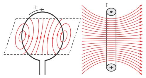
*Figure 53: The "spin rule" magnetic field lines* The direction of magnetic field lines "twist rule"
