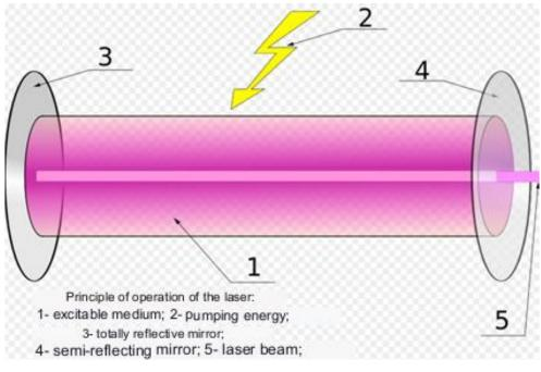
Figure 93: Laser operating principle
