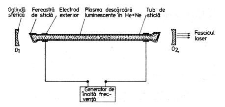
Figure: the main elements of a laser with a mixture of helium and neon
