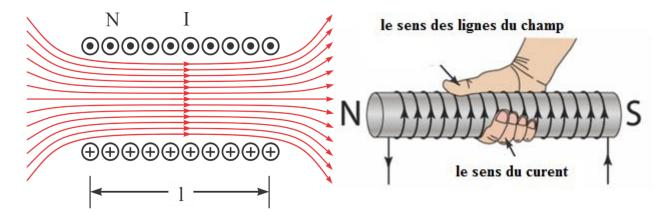
*Figure 55: The direction of the field lines and the direction of the curent.*
