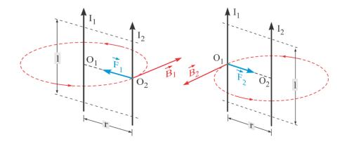
Figure: 66: Magnetic interaction of electric currents
