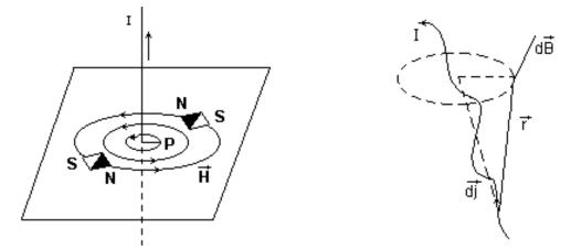
Figure 70: Magnetic field created by the wired conductor traversed by an electric current
