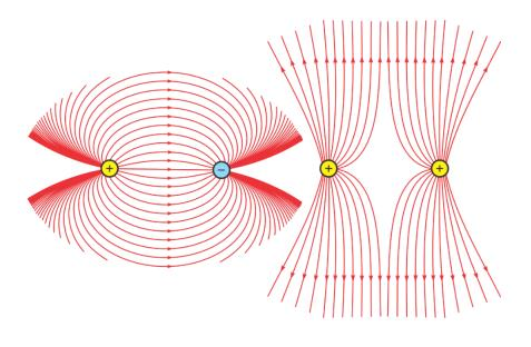
A B Figure 8: A: Power lines of a pair of point charges of opposite sign; B: Electric lines of a pair of point charges of the same sign
