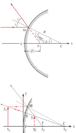
The focus of a convex mirror is virtual (it forms at the extension of the real rays).
