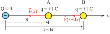
Figure 10: Electric charges and forces (Q < 0)
