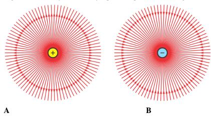
Figure 7: A: The field lines of a positive point-like charge; B: Field lines for a negative point charge
