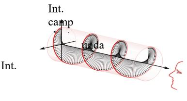
The circularly polarized wave can have two directions of rotation: the dextrorotatory direction and the levorotatory direction.
