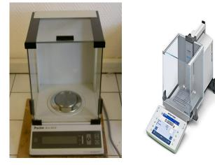
**The principle of operation** of these balances is based on the variations in the electrical characteristics of certain materials when they are subjected to mechanical compression.
