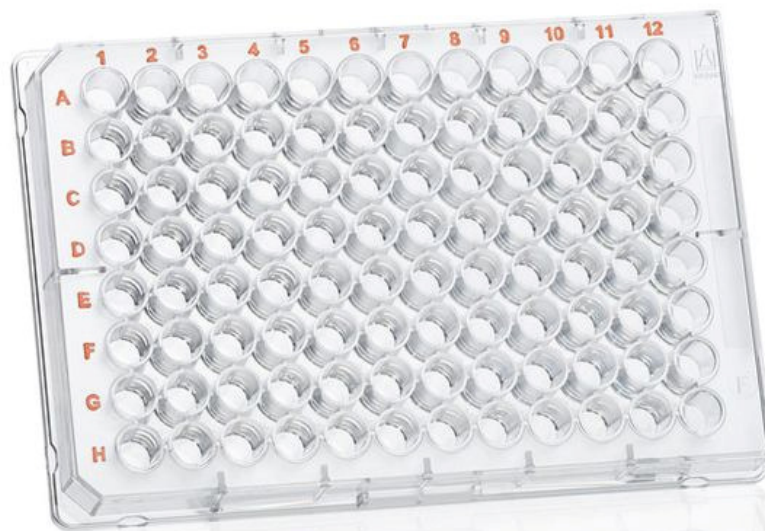
Figure 2.10. 96-well plate for minimum inhibitory concentration testing (URL 10).
